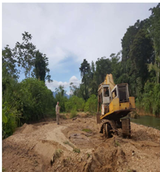
Gravel mining directly from riverbed
